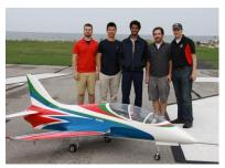
The Ohio State University team launched the Avanti JetCat UAS from Kelleys Island in Lake Erie on August 30. The UAS immediately went into autonomous mode and then made two passes over the 15-kilometer course, at an average speed of 147 mph. The JetCat weighed 68 pounds at takeoff, has an 8-foot wingspan, and is equipped with a turbojet engine rated at 40 pounds of thrust.
